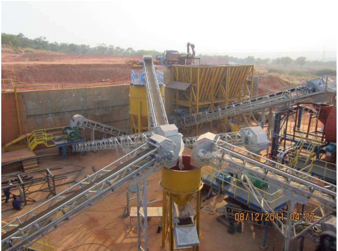
View of the conveyor feeding the scrubbers
